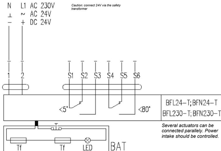
Connection diagram for actuators BFL24-T, BFL230-T, BFN24-T, BFN230-T.
