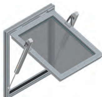
Fig. 65 - mcr OSO THERM 75 smoke exhaust window with two G spindle actuators with shifted pivot point
