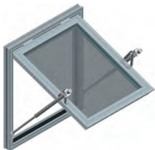
Fig. 101 - mcr OSO THERM 75 smoke exhaust window with two S spindle actuators with shifted pivot point
