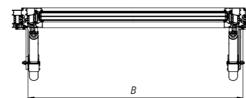
Fig.23 - B-B horizontal cross-section through mcr OSO THERM 75 smoke exhaust window in closed position
